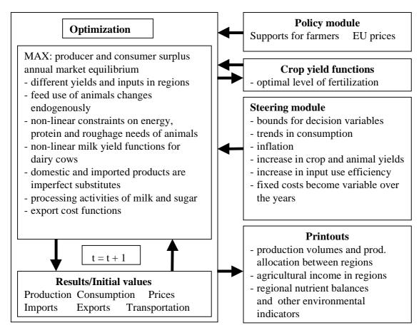
Figure 7A.1 Basic structure of the DREMFIA model
